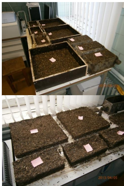
Figure 1. The drying process of the lightweight concrete of the new building material from spropel and hemp shives
