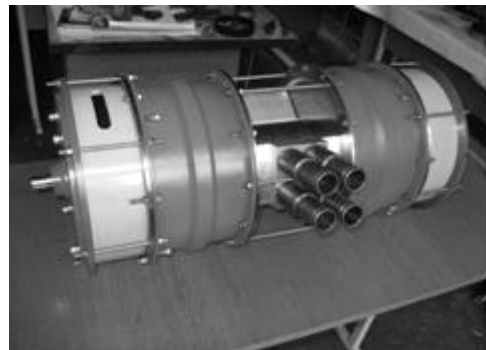
Fig. 1. Rotary-vane external combustion engine.
