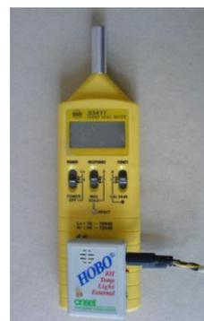
Pic. 1 Sound level meter and Hobo
