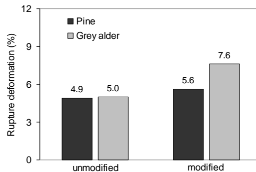
Fig. 2. Rupture deformation of polymer composites filled with initial wood bark and modified ones
