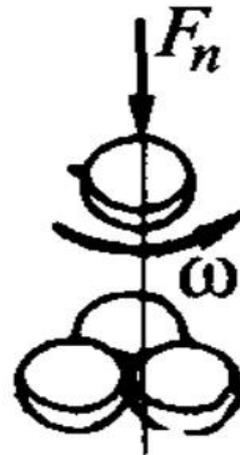
Fig.2. Four-ball test subassemblies principal block diagram
