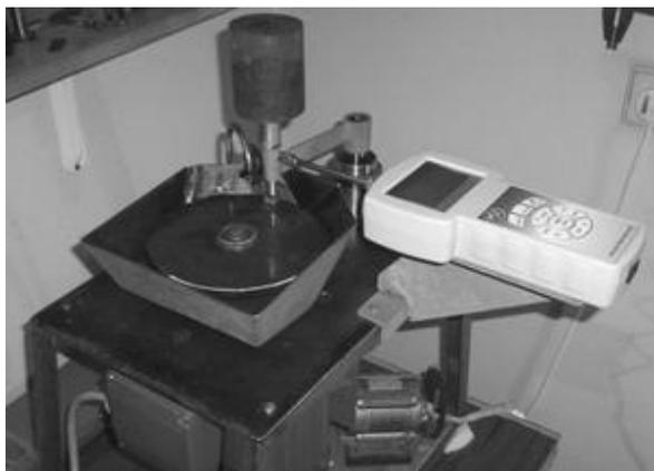
Fig.1 Oil additive testing machine
