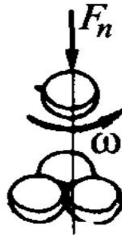
Fig.2. Four-ball test subassemblies principal block diagram
