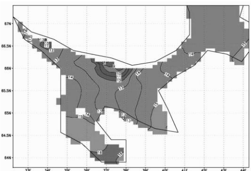
Fig. 9. Surface temperature distribution, 30 years of colder (-1°C) air.
