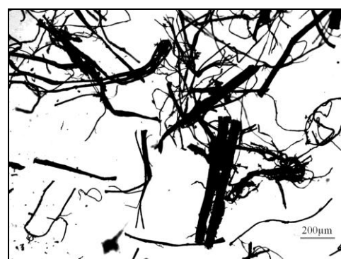
Fig.2. Dew-retted alkaline pretreated, steam explosion treated fiber agglomeration
