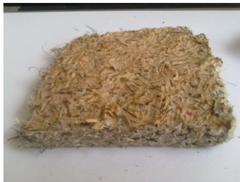
Fig.3. C1 Hemp shive and cellulose composite material
