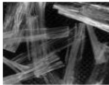
*Fig.4. Fibers of polypropylene
