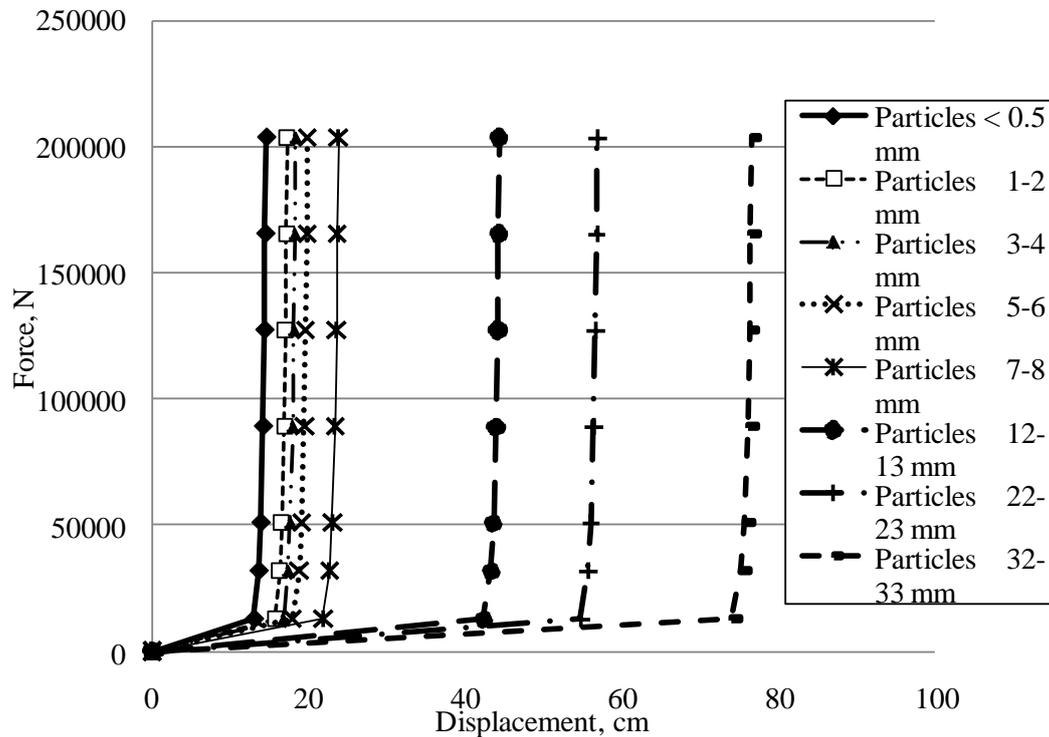
Fig. 2. Force – displacement characteristics of compacting
