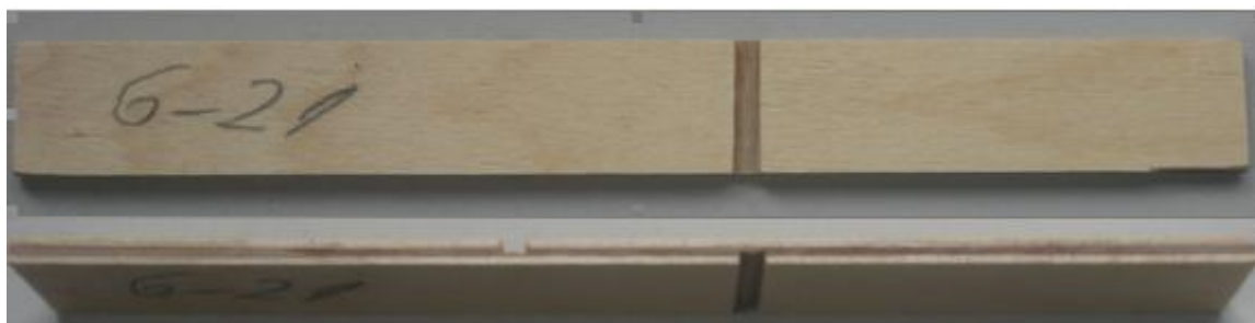
Fig.5. Plywood samples for tension shear test in accordance with the standard EN 314
