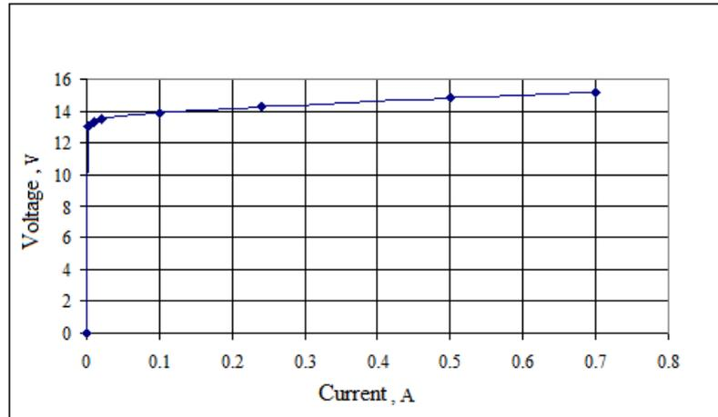
Fig.3. Photo-electric module, power recorders Volt-Ampere characteristic
