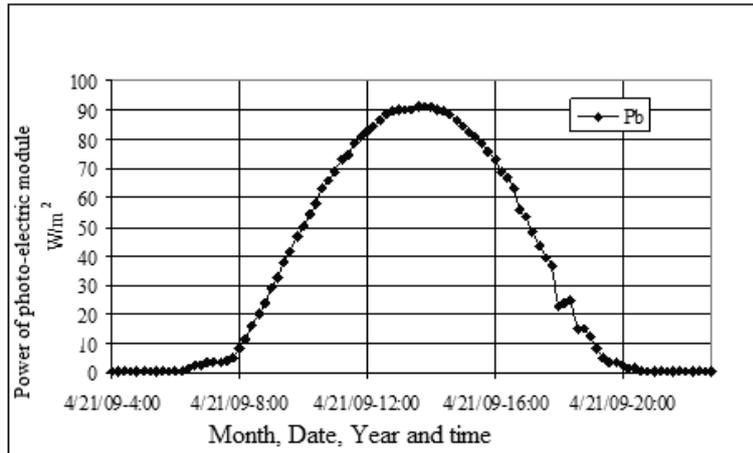
**Fig.4. Photo-electric power module diagram 2009, 21st April**
