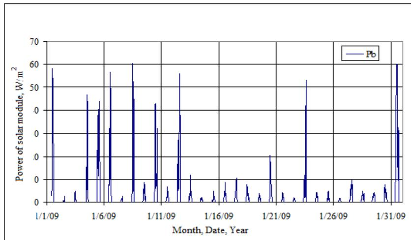
**Fig.5. Photo-electric power module diagram and power diagram energy output in January, 2009<sup>th</sup>**
