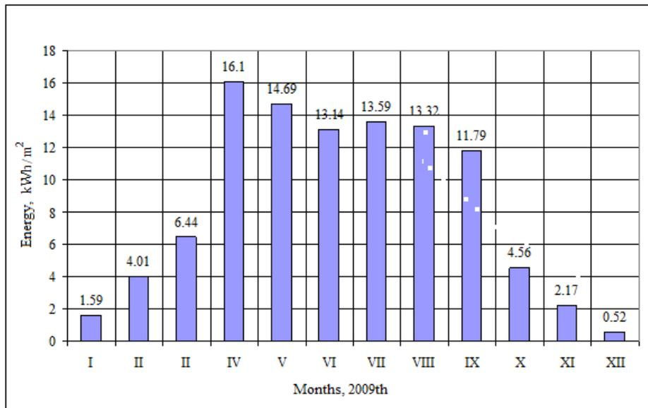
Fig.9. The recorded output (the batteries are not loaded) energy levels in 2009th, Total 101.9 kWh/m<sup>2</sup>
