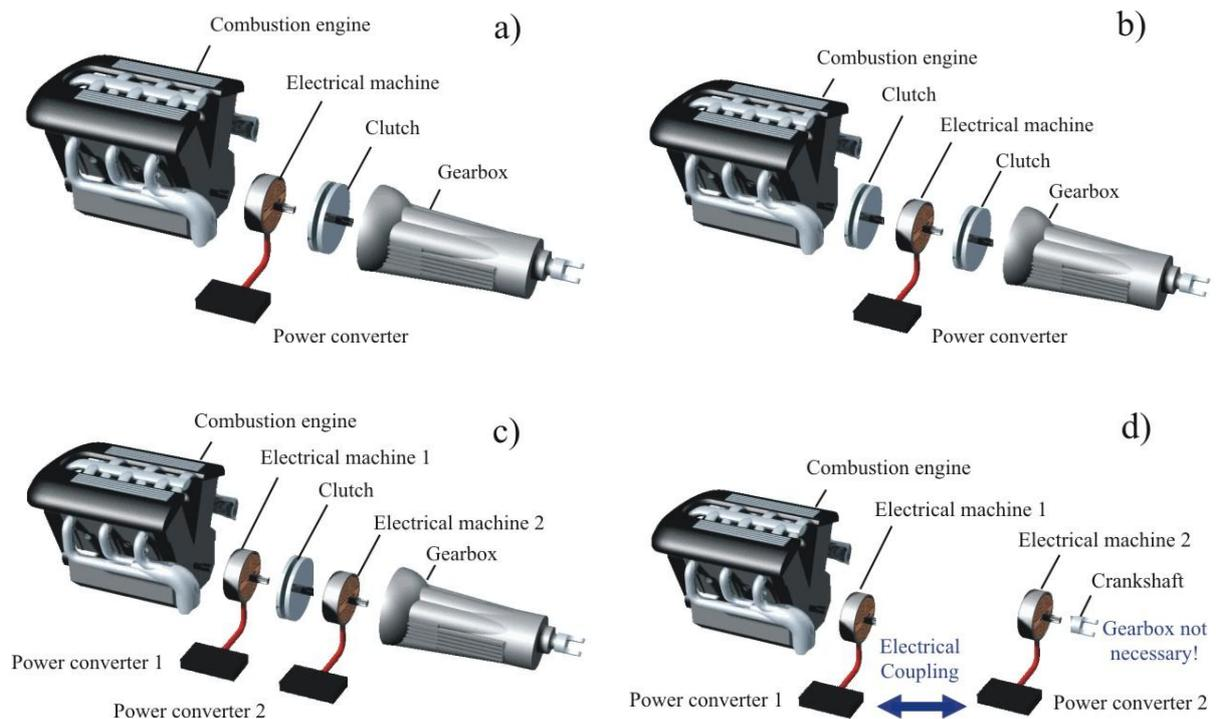
Fig. 1. Power train topologies for hybrid electric vehicles
