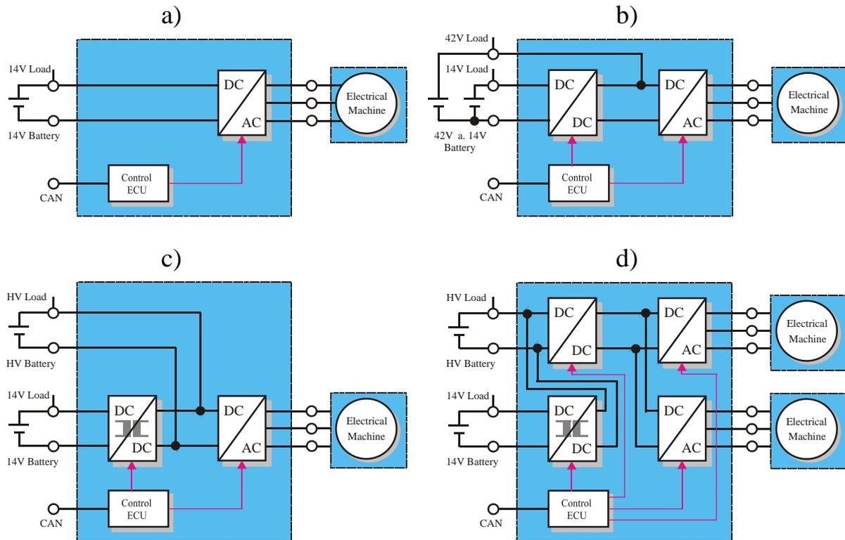
Fig. 2. Electrical system architectures for hybrid electric vehicles
