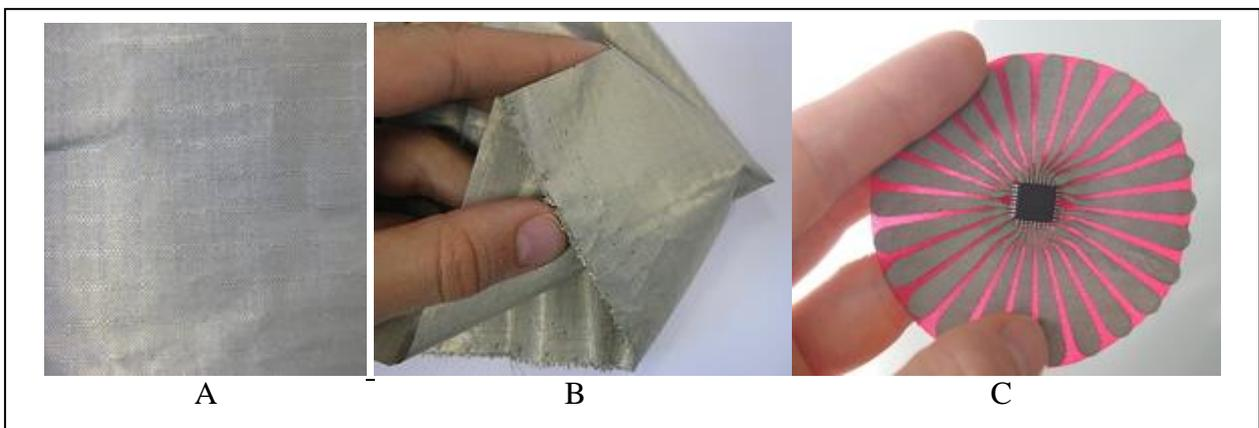
Fig. 2. A, B – Tin/copper coated fabric; C – Conductive fabric stuck to soft circuit
