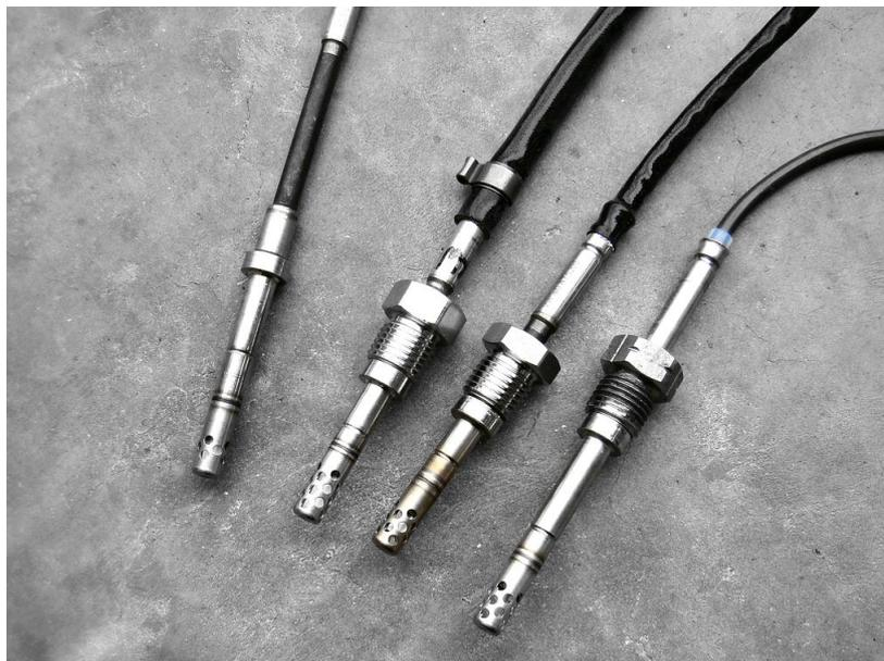
*Fig. 1. Picture of some of the widespread thermal sensors car*
