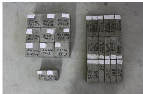
Fig. 1. Specimens containing lamp glass powder
